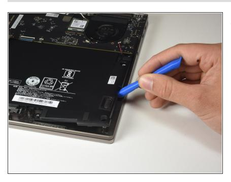
Lift up the speaker with the iFixit Opening Tool and remove the speaker.
