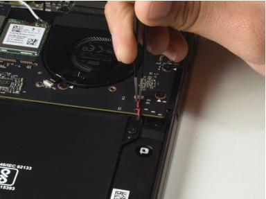
Disconnect the red and black wire from the motherboard to free the speaker.
