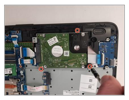
Remove the three 3mm JIS #0 screws from the hard drive.
