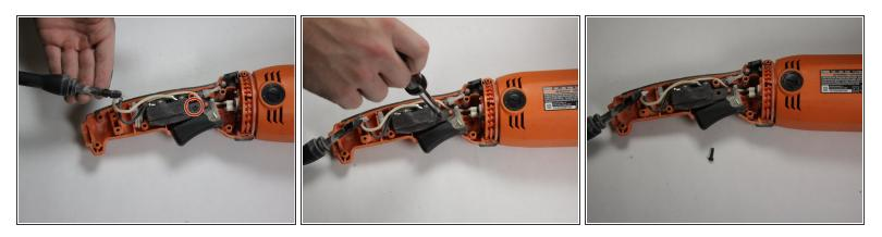
Use a screwdriver to unscrew and remove 1 M4 x 14 mm Screw [23].
