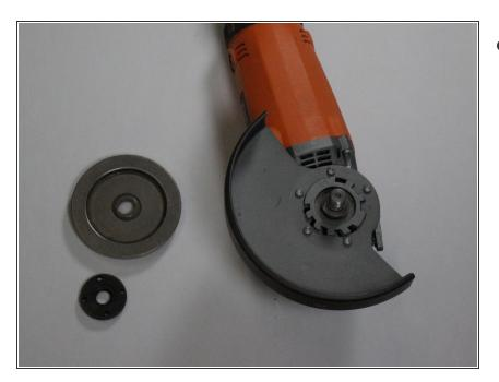
To get to the guard, unscrew and remove the Clamp Nut [34], Grinding Wheel (not pictured) [35], and Backing Flange [36].
