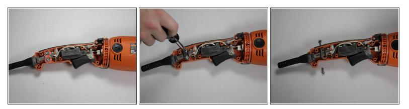
Use a Hex Screwdriver to unscrew and remove the 2 8-16 x 1/2 in. Screws [29].
