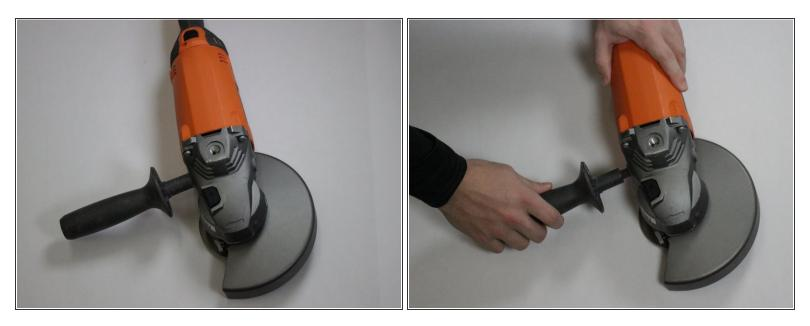
• Take hold of the Side Assembly Handle [8] and unscrew to detach from the grinder.
