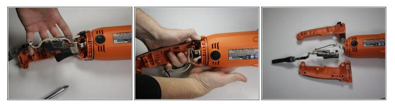
• The whole wiring assembly should be able to be lifted out of where it currently is as seen in the first photograph.
