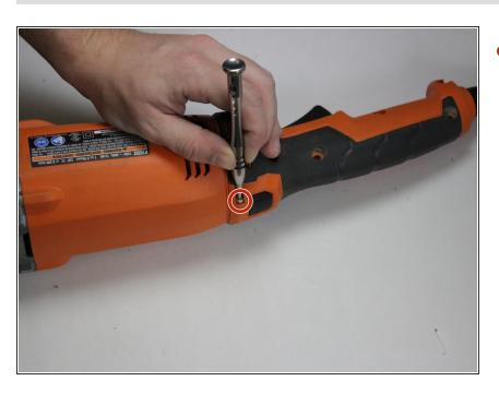
Using a Torx T10 screwdriver, remove the M3 x 10mm screw.
