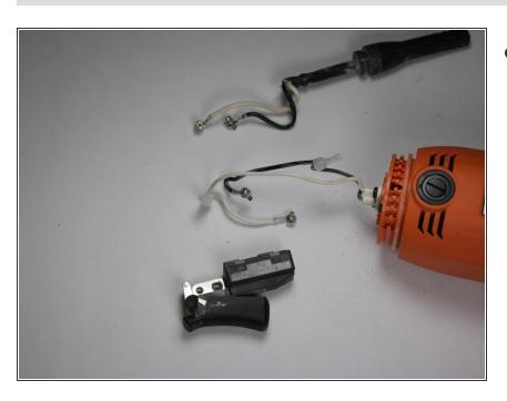
The Switch is now free of the Grinder. Dispose of the broken Switch and install your new Switch.
