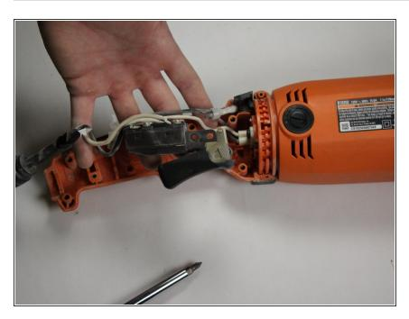
Gently lift away the switch and wires.
