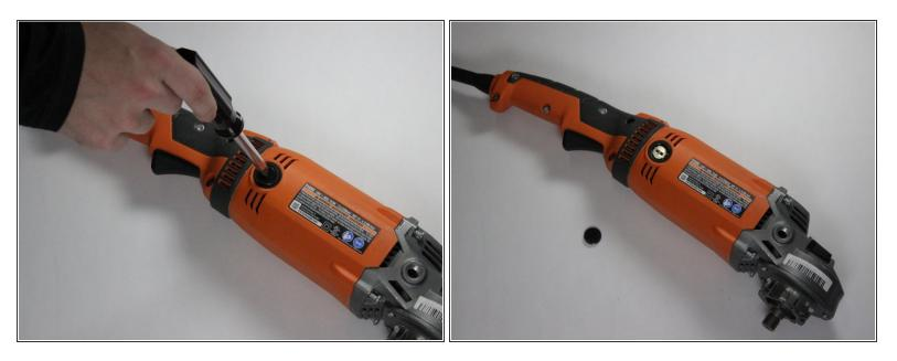
Use a flathead screwdriver to unscrew the brush holder cap.
