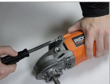
Using a T25 Torx screwdriver, unscrew the four M5 X 28mm Torx screws.
