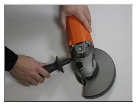
Unscrew the side handle assembly from the gear housing assembly by hand.
