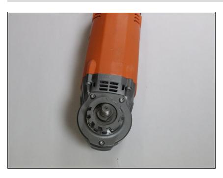
Lift the guard away from the output shaft assembly.
