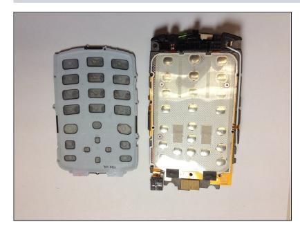
Here is the rubber keyboard and the dome switch circuit board. A quick inspection of these elements can reveal keypad malfunctions. Look for dirt or debris that do not belong there.
