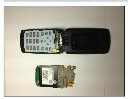
• Here is the phone without the dome switch circuit board.
