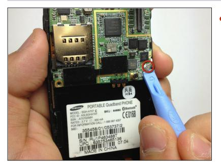
• Use the prying tool to disconnect the small connector.
