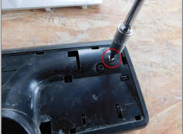
Unscrew both Philips screws from the top of the brush.
