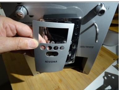
Remove the plastic plate with the 'Nivona' label carefully with a plastic opening tool.
