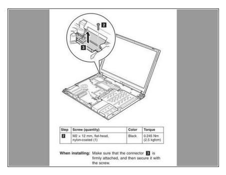
Verify LCD Assembly Connector is clean, not damaged and connected properly.
