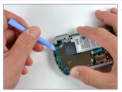
Use a plastic opening tool to gently flip up the left trigger connector.
