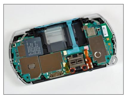
Remove both headphone jack and analog joystick screws using your #00 Phillips screwdriver.
