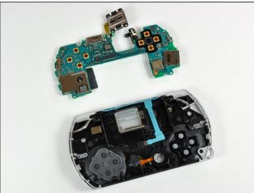
Use a plastic opening tool to disconnect the display cable from the logic board.
