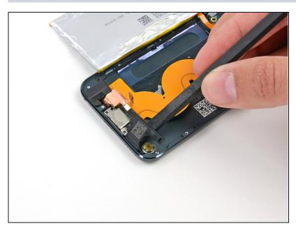
Use the flat end of a spudger to pry the speaker up from the rear case.
