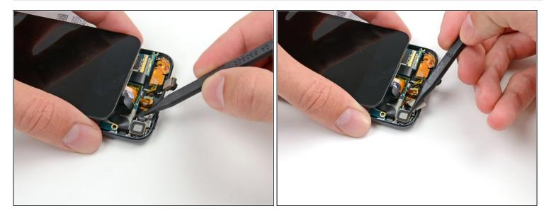
• Use the tip of a spudger to gently pull the rear-facing camera ribbon cable out from underneath the logic board.
