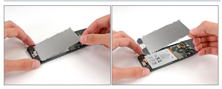
• Lift up and remove the LCD plate from the iPod.
