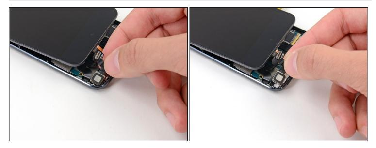
• Lift the rear-facing camera up out of its socket and remove it from the iPod Touch.
