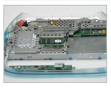
Remove the two small Phillips screws from the RJ-11 board.
