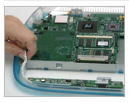
Disconnect the charger board cable from the logic board.
