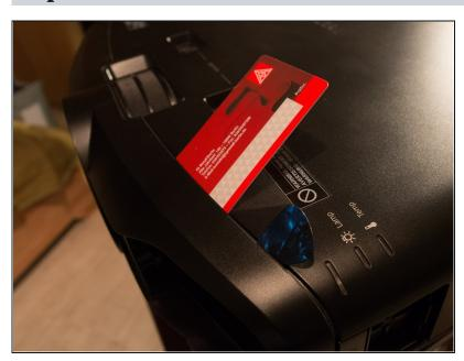
You can take of the front now. I used a guitar pick and a plastic card. Insert the pick carefully in the left side of the projector between case and front plate and try to make your way to the middle. Do the same from the right side, the front cover should come off now.
