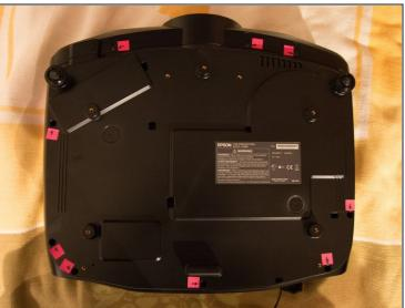
Remove 10 non metric screws, one inside the lamp housing and 9 at the bottom. I
