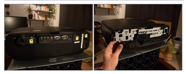
Remove the metric screws at the back, I marked them with yellow markers. The rear plate should come off than
