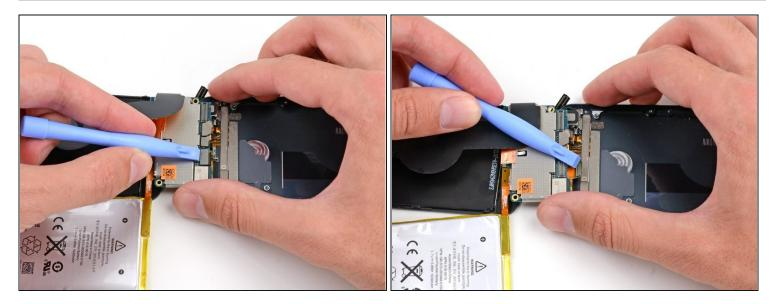
• Use a plastic opening tool to disconnect the display cable from its socket in the logic board.
