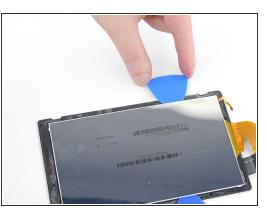
Continue sliding the opening pick along the bottom edge to slice the adhesive.
