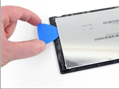
• Insert and slide the opening pick along the left edge of the screen assembly to slice the adhesive.
