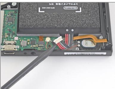
Use the point of a spudger to pry the battery connector straight up and out of its socket on the motherboard.
