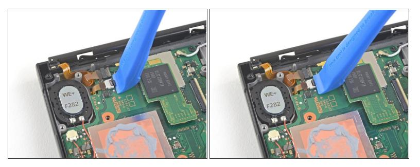
• Use an opening tool, spudger, or your fingernail to flip up the small, hinged locking flap on the smaller LCD ribbon cable ZIF connector.
