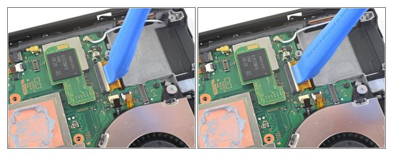
• Use an opening tool, spudger, or your fingernail to flip up the small, hinged locking flap on the LCD ribbon cable ZIF connector.
