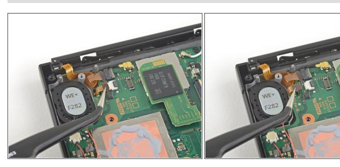
Use a pair of tweezers to pull the ribbon cable straight out of its connector on the motherboard.
