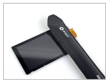
Heat the right edge of the screen assembly for around two minutes to help soften the adhesive.
