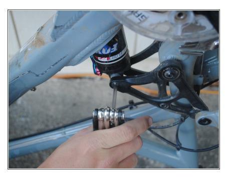
Remove the 40mm screw that connects the shock to the link arm of the suspension.
