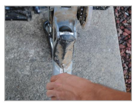
Remove the 10mm screw and take the bash guard off of the frame.
