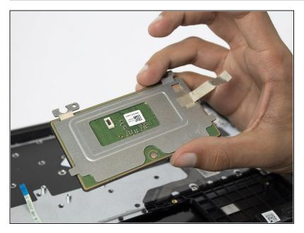
Carefully remove the trackpad from the computer.
