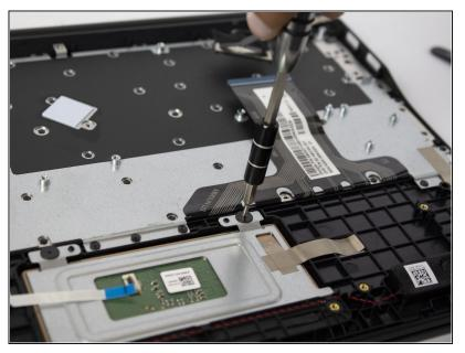
Using the Phillips Head Screwdriver, remove the screws at the topmost part of the panel holding the trackpad in place.
