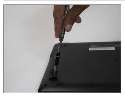
• Unscrew the screws with the Phillips #00 screwdriver.
