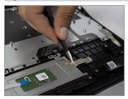
Using <u>tweezers</u>, remove the silver electrical tape.
