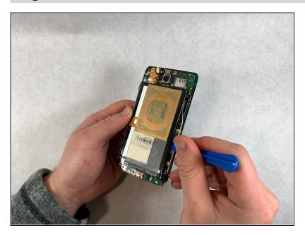
Gently pry the motherboard out of the frame using the plastic opening tool.
