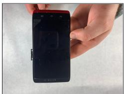
• Gently remove the SIM card tray from the device using a spudger.
