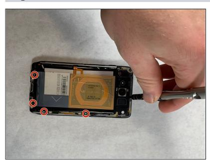
Remove the four T5 Torx screws securing the motherboard.
