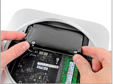
Pull the hard drive away from the front edge of the mini and remove it from the outer case.
