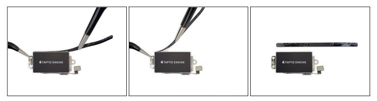
Peel up and remove the plastic bumper strip from the Taptic Engine.
