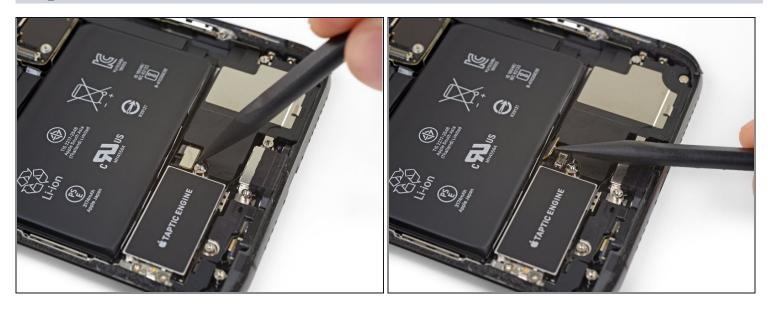
• Use the tip of a spudger to pry up and disconnect the speaker connector.
