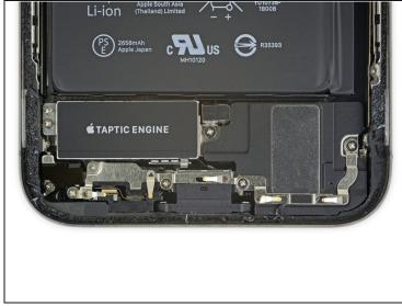
• Remove the five 1.4 mm tri-point Y000 screws securing the bracket below the Taptic Engine and main speaker.
