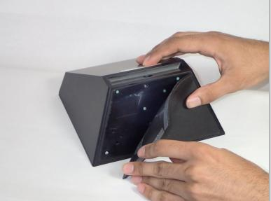
After the protector has been removed, use your hands to gently remove the taped-in rubber foot from device.
