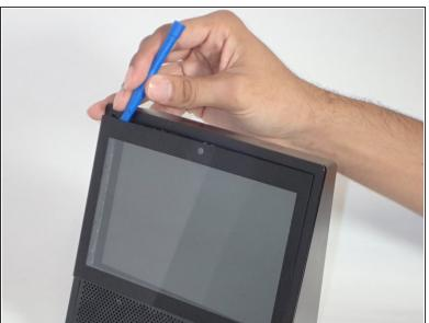
Use the plastic opening tool to gently lift the plastic protector from the screen.
