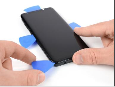
Insert a fourth opening pick at the left side of the frame and slide it down to the bottom left corner to cut the adhesive.
