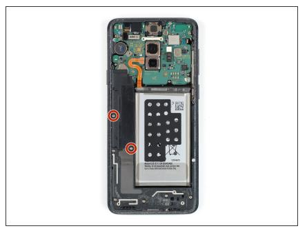
Remove the two 4 mm Phillips #00 screws.
