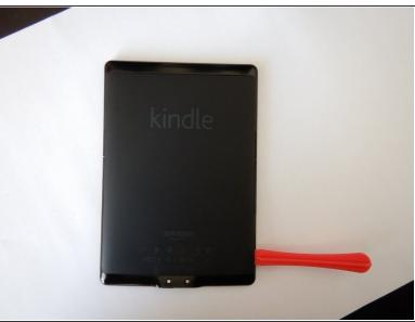
Use plastic opening tools to pry open the case starting on the long side. The cover has a total of 8 clips, 4 of which (located on the long sides) are designed so they will be damaged when the device is opened.
