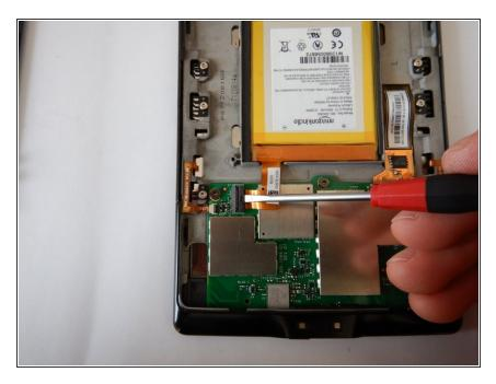
Then carefully disconnect the battery flex cable, ensuring that the contacts are not being shortcircuited.
