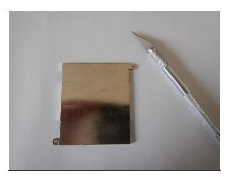
Remove any adhesive residue from the battery cover and the housing cover with a scalpel / rubbing alcohol.
