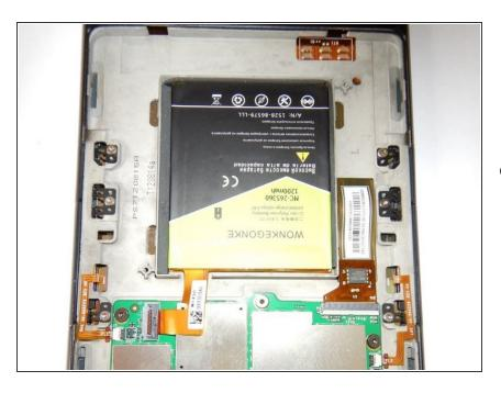
The new battery can be fastened through the remaining adhesive residue. Reconnect the flex cable of
