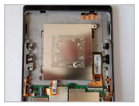
Remove the two TX5 screws from the battery cover.
