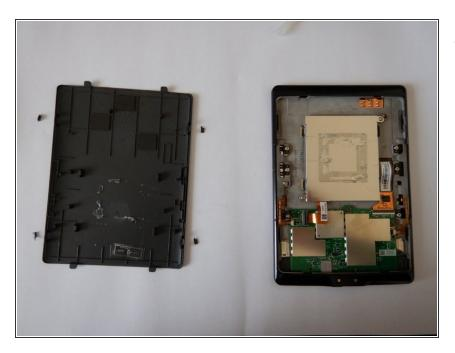
After loosening the adhesive, the case cover can be easily removed.
