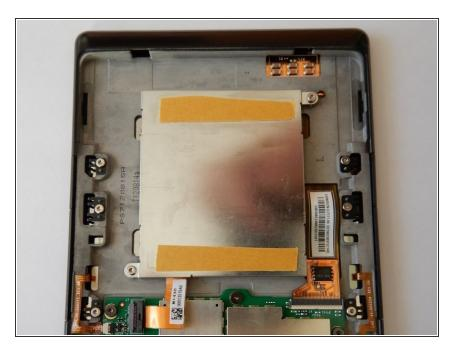
Secure the battery cover with the two TX 5 screws. Ensure a good fit of the back cover with a few strips of double-sided tape. Limit the amount of tape so as not to hinder future disassembly.
