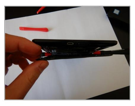
After prying open 3 sides of the cover, it is still attached to the aluminium cover by double-sided adhesive tape. Use a screwdriver to create a small gap and use the scalpel to cut the adhesive. Alternatively you can losen the adhesive with a heat gun.
