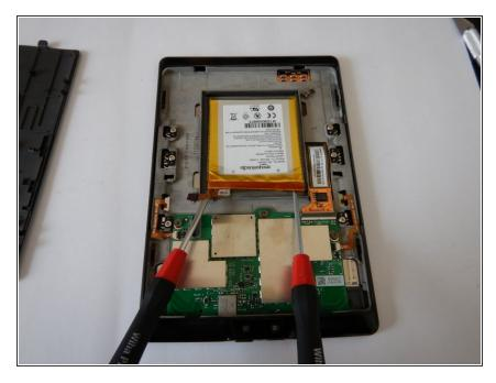
The battery is adhered to the housing, it takes some force to remove it. Avoid puncturing of the battery as it could catch fire and/or explode! Dispose of the old battery properly.
