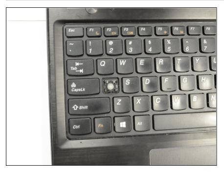
To replace the key, place the key above its mechanism and gently press it into place.
