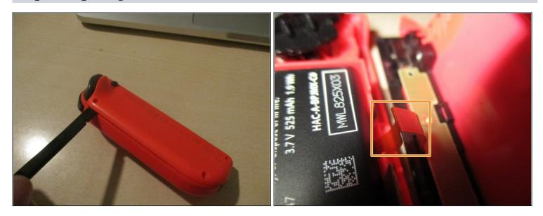
• Insert the flat side of a spudger on the curved side to pry the back cover open
