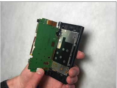
Wedge a plastic opening tool under the bottom of the circuit board and push upward to separate the circuit board from the back of the phone.
