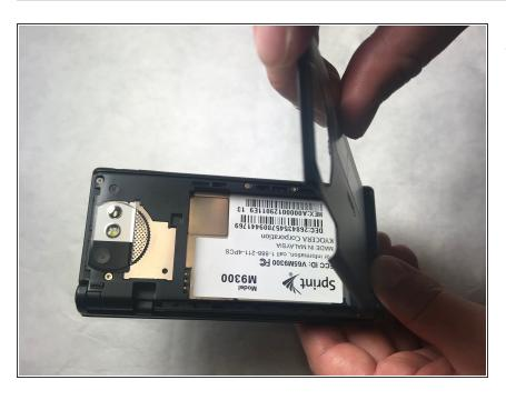
Pull up on the back cover and lift the top to separate it from the phone.
