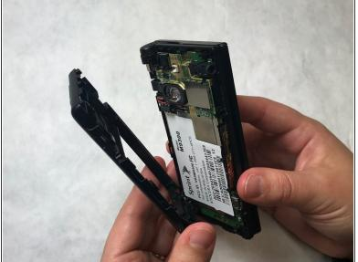
Wedge a plastic opening tool under the black outer casing of the phone. Push the plastic opening tool down and outward while rotating the phone to pry the black outer casing off.
