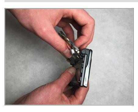
Push the camera gently out of its housing towards the side of the circuit board it is connected at to dislodge it.
