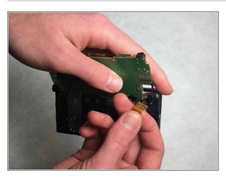
Grasp and pull up on the 32 pin connector attached to the circuit board to remove the camera.
