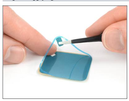
Use a pair of tweezers to carefully remove replacement adhesive with the blue protective film from the backing paper.
