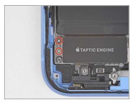
Remove the two 1.8 mm Phillips screws securing the Taptic Engine.
