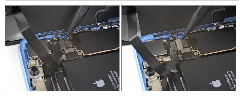
• Use the tip of a spudger to pry the front sensor assembly connector up from its socket.
