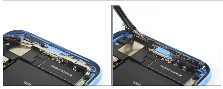
• Lift the bracket from the edge nearest the battery. Don't try to fully remove it, as it's still connected via a small flex cable.
