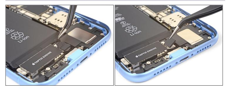
• Remove the piece of black tape and the small rubber rectangle covering the Taptic Engine connector cover.
