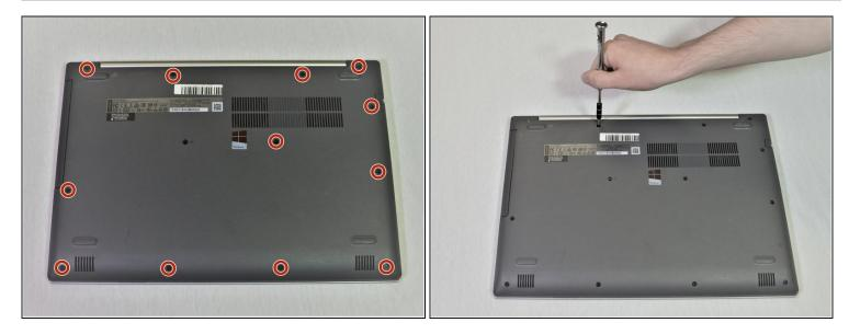
Using the Phillips #1 screwdriver, remove the twelve screws around the back panel from the laptop.
