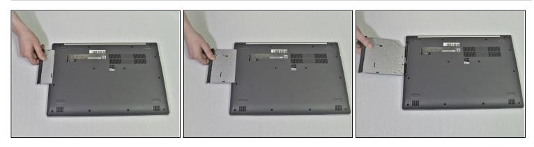
• Carefully remove the optical drive bracket by pulling the bezel away from the laptop.
