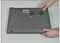
Use an opening tool to pry out the back cover.
