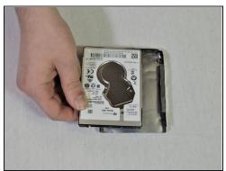
• Detach the bracket from the hard drive by pulling the bracket edges apart.
