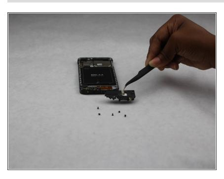
After checking for debris and water surrounding the speaker area, replace with new speaker.
