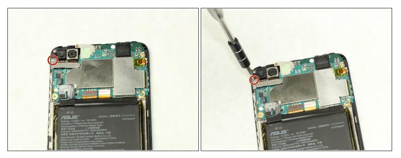
Using a removable head screwdriver and a PH0 bit, begin removing the panel beneath the two cameras by unscrewing the screw.
