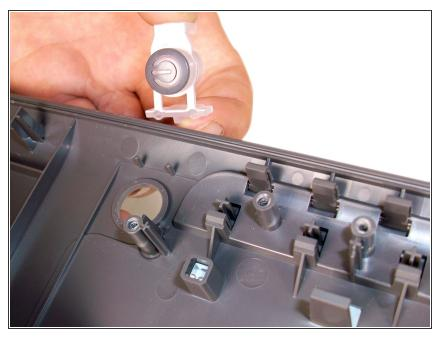
The power button is not clipped in and should easily slide off of the plate once the button circuit board is removed.
