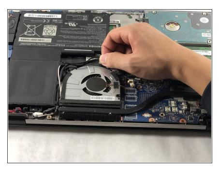
Gently disconnect the fan cable from the device.
