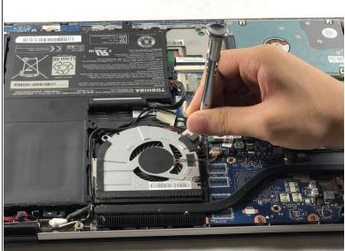
Remove the two 5 mm screws using a Phillips #1 screwdriver.
