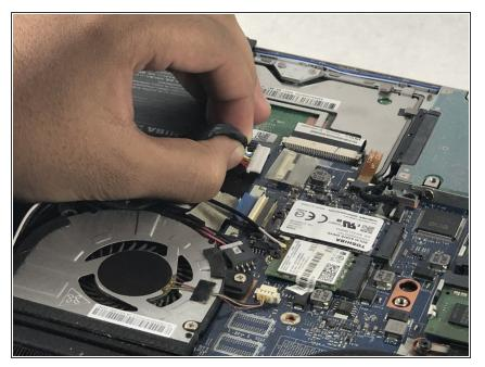
• Disconnect the battery connector from the motherboard.
