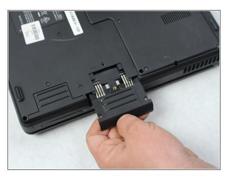
Gently slide the hard drive away from the computer using the built in ridges.
