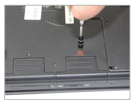
Once you have located the hard drive, you will then need to remove the 3 mm screw using the Phillips #1 screwdriver.
