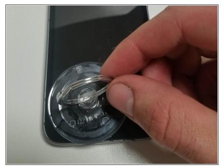
• Place the suction cup tool on the bottom left corner of the screen.
