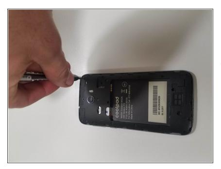
Using a Phillips #000 screwdriver, remove the screws holding the rear mid-frame cover to the mid-frame assembly.
