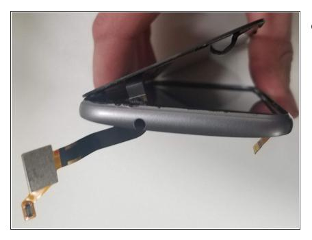
Once the screen is free from the adhesive, slide the flex cable through the middle chassis assembly.
