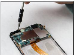
• Using the screwdriver with the PH0 bit, unscrew all screws found on the circuit board.
