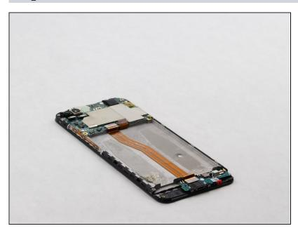
• Remove the battery and replace it with the new battery.
