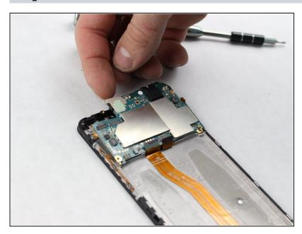
• Gently lift and remove the circuit board.
