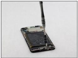
• Once the back has been removed, you will need to unscrew the four screws on the bottom panel with an AT3 bit.
