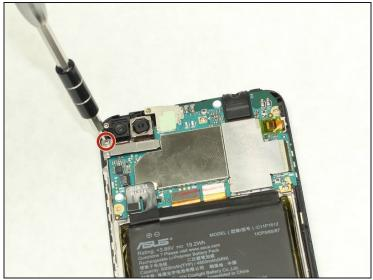
Using a removable head screwdriver and a PH0 bit, begin removing the panel beneath the two cameras by unscrewing the screw.
