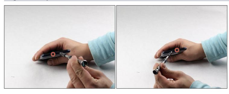
• Using a removable head screwdriver and a T3 bit, begin by removing the two screws located on either side of the charging port.
