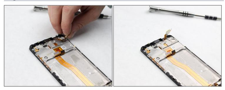
• Disconnect the power cable on the right side of the device and leave it hanging in place.
