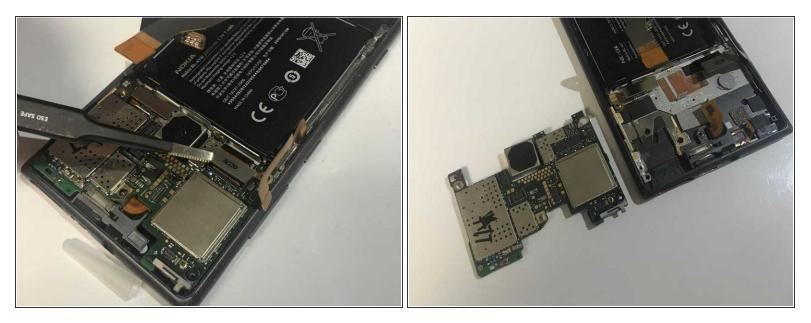
• Remove the motherboard by sliding tweezers between it and the back of the screen. Lift up.
