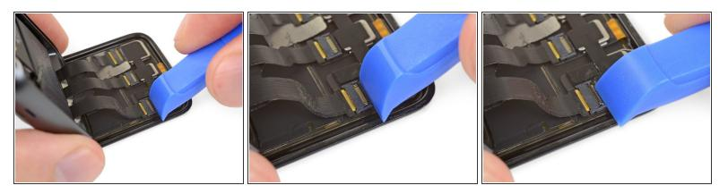
• Carefully use a pry tool or a clean fingernail to unlock the first of the three <u>ZIF</u> connectors by prying up the small black locking flap opposite the cable.
