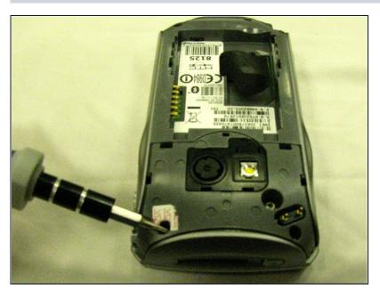
Remove the four black Torx head screws in each corner.
