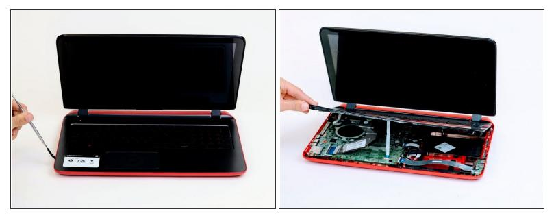
• Flip computer over and wedge metal spudger along the computer to pop off keyboard panel
