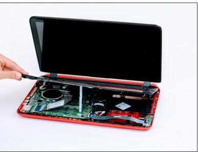
Flip computer over and wedge metal spudger along the computer to pop off keyboard panel
