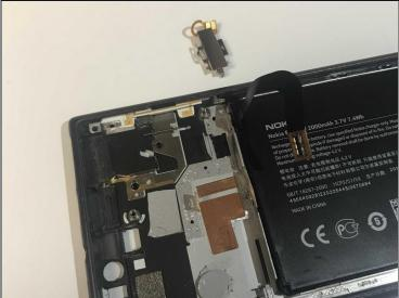
Pry off the metal vibrating unit using tweezers.
