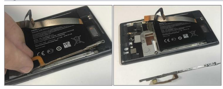
• Carefully pull the metal rod out.
