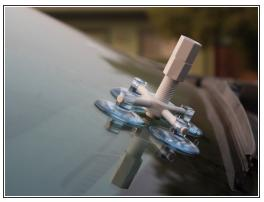
• To attach resin chamber, screw the chamber into the center ring of the applicator base.
