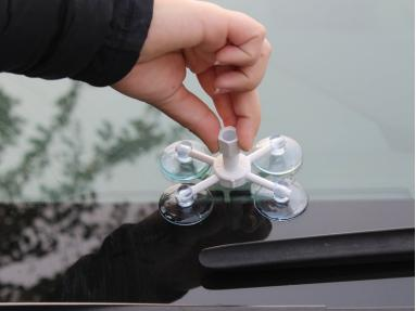
Once finished curing, remove the resin chamber and the pressure driver by screwing counter clockwise.
