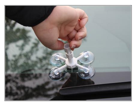
Screw the resin chamber clockwise until it is in contact with the windshield.
