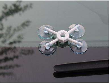
Attach the Rain-X applicator base to the windshield, with the center of the base directly above the chip.
