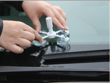
Remove the applicator by using the tabs on the suction cups.
