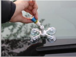
Apply 3-6 drops of resin from the resin repair bottle into the resin chamber.
