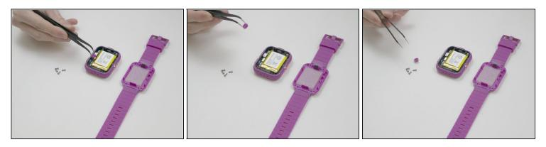
• After removing the backplate, lift the master switch up from the circuit board.
