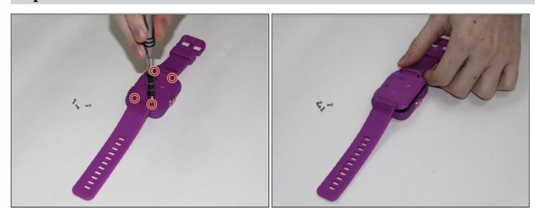
• Next, use the Phillips #00 screwdriver to unscrew the four 6.0 mm screws located in each corner of the watch to remove the backplate.
