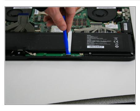
Use an opening tool to unlock the ZIF connector securing the white ribbon over the battery.
