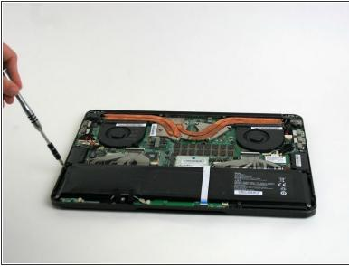
Remove the seven screws holding the battery in place using a Phillips #0 screwdriver.
