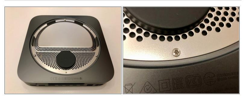
● The lid is secured with the same TR6 screws as the 2014 model
