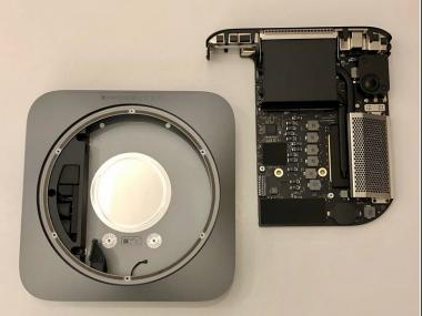
• Slide the motherboard out by gently applying pressure to the heatsink
